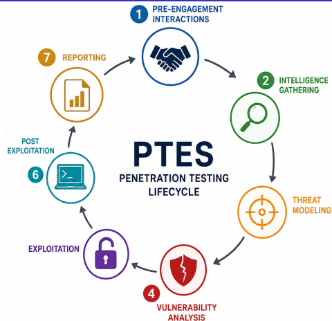
Abb. 1: The seven phases of the Penetration Testing Execution Standard, executed iteratively until the engagement objectives are met. Rechte s. Anhang.
