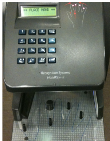
Fig. 2: Device for reading hand geometry.
